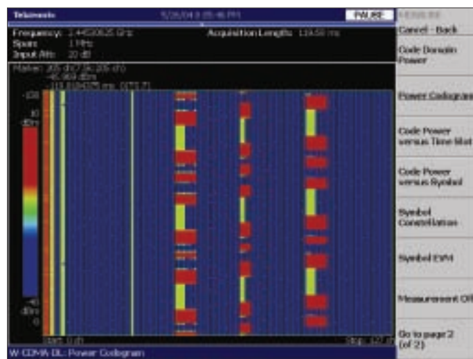
Figure 3-20. Codogram measurement of W-CDMA compressed mode.
