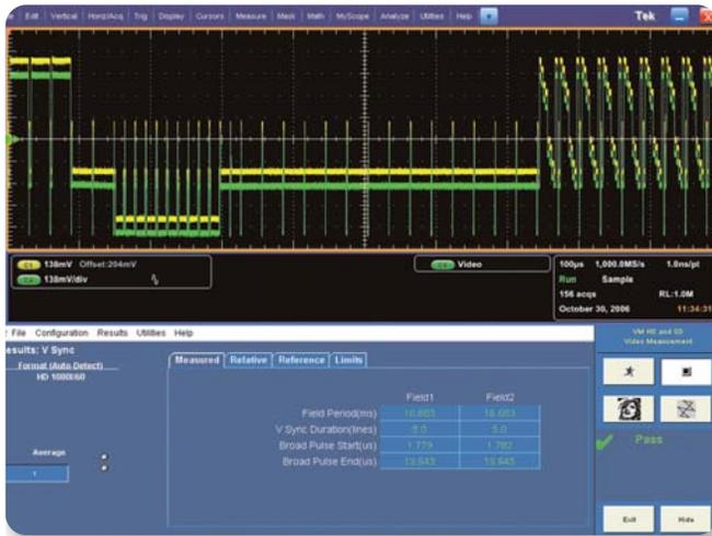
► **Figure 24.** VM6000 Vertical Sync measurement results for an HD signal.
