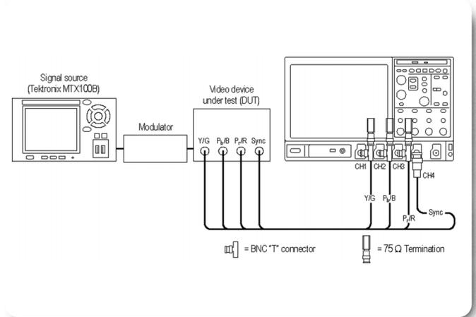
► **Figure 4.** Component connection with separate sync.
