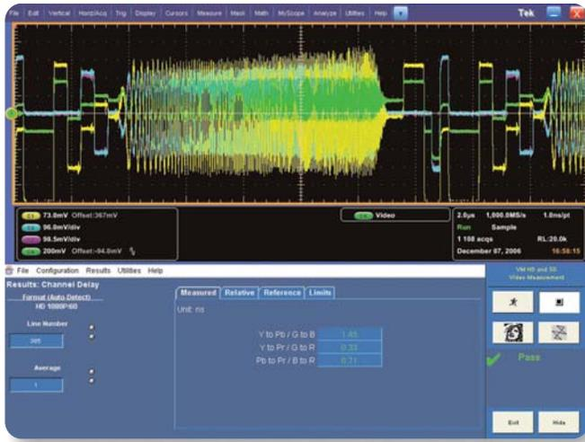
► **Figure 20.** Channel Delay measurements.
