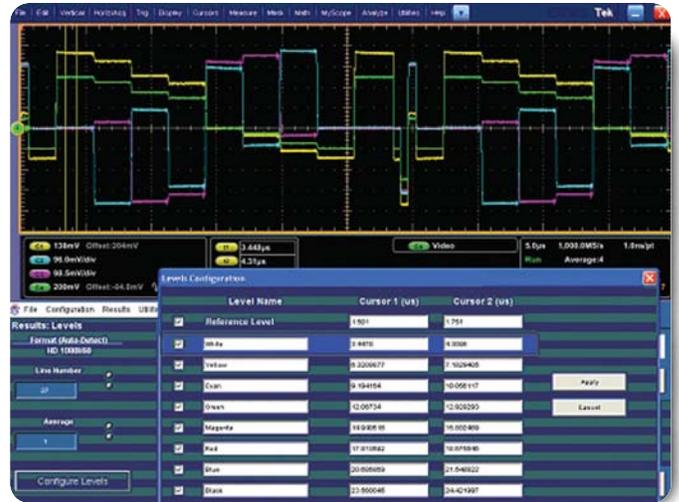
► **Figure 12.** Custom timing configuration of VM6000 Levels measurement.
