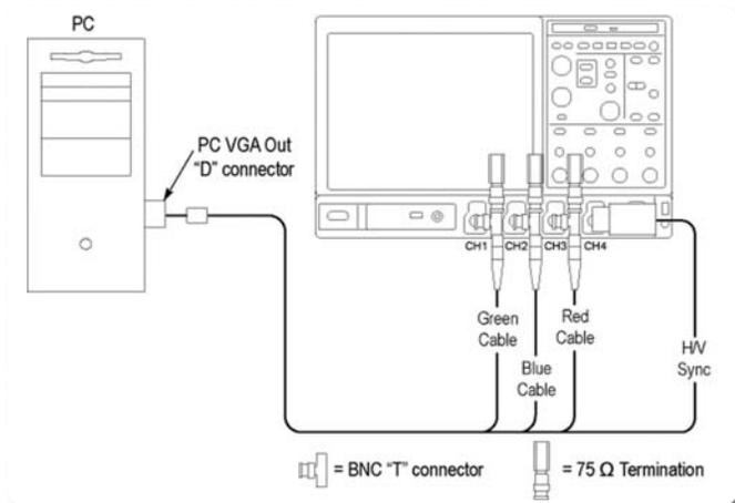
► **Figure 5.** PC VGA connection to instrument.
