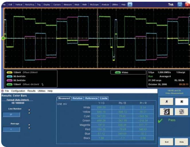
► **Figure 8.** Color Bars measurement display.
