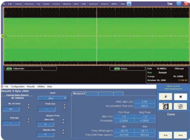
► **Figure 28.** VM6000 Horizontal Sync Jitter measurements.
