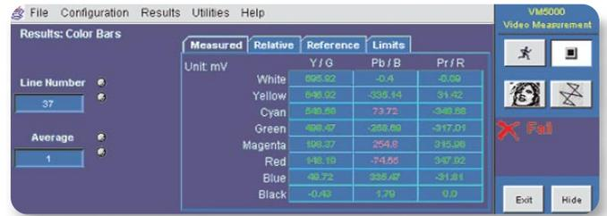
► **Figure 31.** Pass (green) or fail (red) limits testing of a Color Bars signal.
