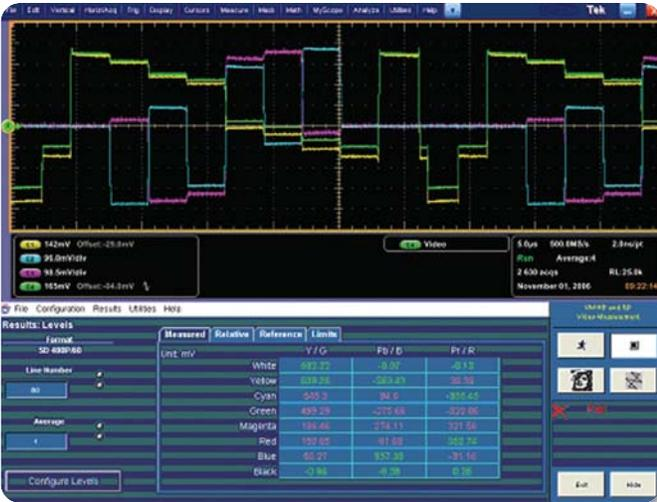
► **Figure 11.** Levels display of an SD signal with HD colorimetry.
