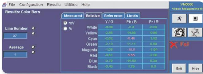
► **Figure 30.** Relative to reference results for a Color Bars signal.
