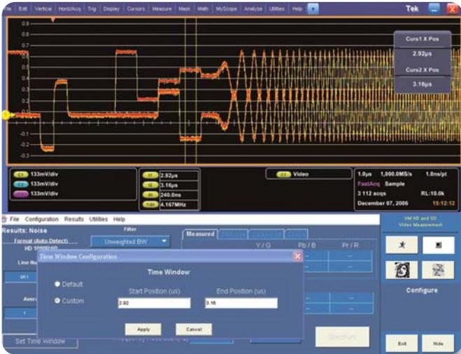
► **Figure 18.** Set time cursors can define Noise measurement interval in a complex signal.
