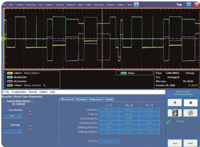
► **Figure 26.** VM6000 Short Time Distortion measurements
