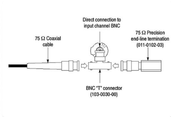
► **Figure 6.** Termination at input to instrument (VM6000 shown).
