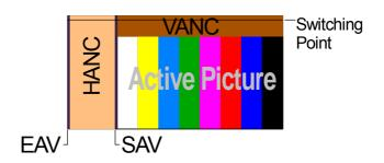
Ancillary data packets should not be located in the lines identified as a switch point – defined by SMPTE RP 168.
