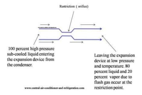
The general principle behind any metering device is it acts as a restriction. You can see it in the diagram above. It reduces high-pressure, high temperature refrigerant from the condenser liquid line to low-pressure, low temperature refrigerant for the evaporator.
