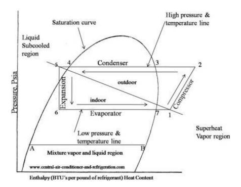
The Ph chart graphically shows where the physical states of these five mechanical components is and what is happening to the refrigerant within these components.
